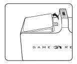
2 Add water to fill-line indicated on label within the reservoir. DO NOT OVERFILL. Add ice to top of reservoir.
